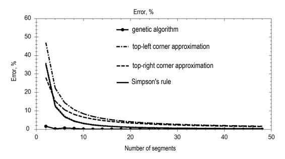
Fig. 5. A result's precision given by genetic algorithm and by numerical methods
