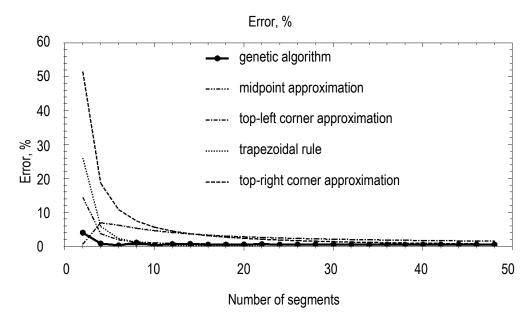
Fig. 11. Results given by the genetic algorithm and numerical methods
