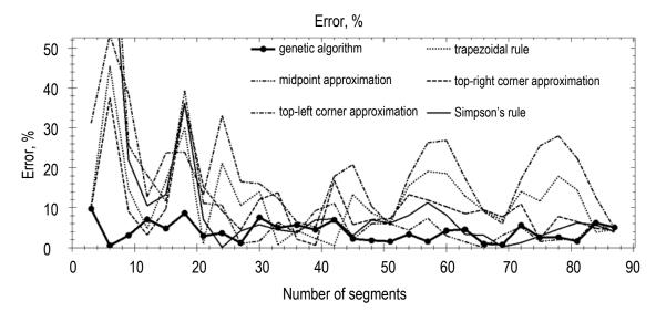
Fig. 12. Results given by the genetic algorithm and numerical methods in case of quickly oscillating integrand In this example we calculated the integral with quickly oscillating integrand
