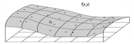
Fig. 8. Diagram of function f(x,y), the partition of the rectangle and chosen points  $c_{ii}$
