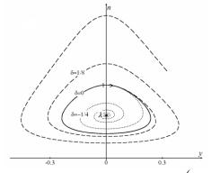
Figure 1. The trajectories (7) on plane (y,n) for  $\lambda = 3/4$ , initial conditions  $y_0 = 0$ ,  $n_0 = 1$  and different  $\delta$ .
