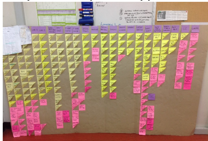
Figure 4: Visual TPM planning. Yellow notes signify standard maintenance and purple notes signify improvements. Folded notes signify completed maintenance.
