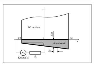
Figure 1. Excitation of ultrasound by a wedge-shaped transducer.
