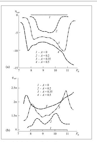
Figure 6. Optimal values of mismatch parameter  $\eta_{opt}$  (a) and Raman-Nath parameter  $q_{opt}$  (b) as a function of the acoustic frequency.
