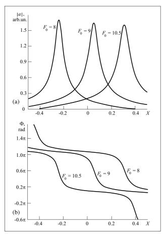
Figure 3. Distribution of acoustic amplitude (a) and phase (b) along the piezoelectric wedge-like plate.
