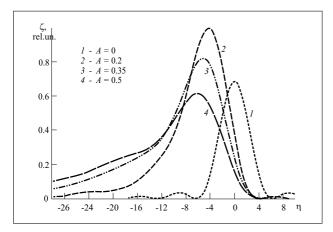
Figure 5. Diffraction efficiency  $\zeta$  as a function of the mismatch parameter  $\eta$ .
