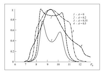
Figure 4. Frequency characteristics of the wedge-shaped transducer with an additional inductance.
