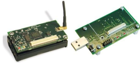
Figure 6: Crossbow Technology Inc. MICAz mote and MIB520CB base station
