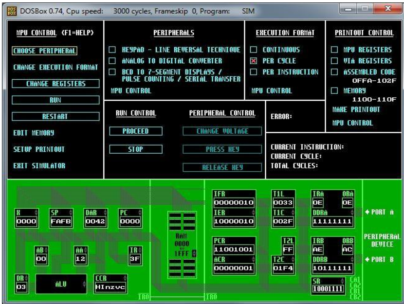
Fig. 1. Main screen of the Graphical 6800 Simulator in DOSBox 0.74
