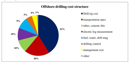
Fig. 5. Typical offshore drilling cost structure.
