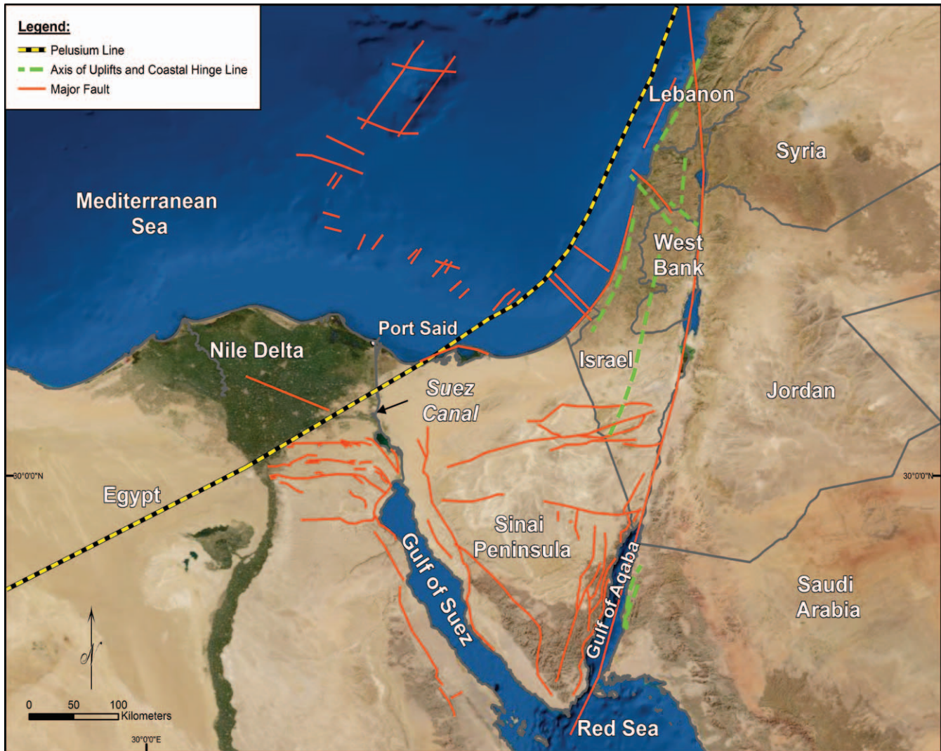
Figure 5. Generalized regional tectonic setting of the Suez Canal, showing some major tectonic elements. The Pelusium Line, which has functioned mostly as a transcurrent fault, lies some 60 km offshore Israel and crosses the Suez Canal south of Port Said, passing along the SE flanks of the Nile Delta and into the Western Desert of Egypt. Some major faults on land and offshore, as well as the axes of major uplifts and coastal hinge lines, are indicated as features that contribute to tectonic instability in the region. (Based on a more detailed map by Neev, 1975).
