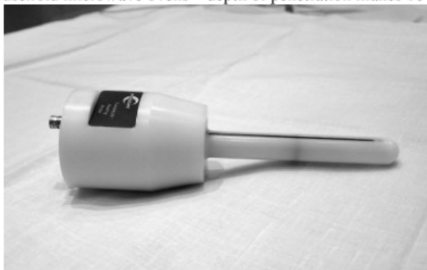
Figure 3. Spiral urological electorde.
