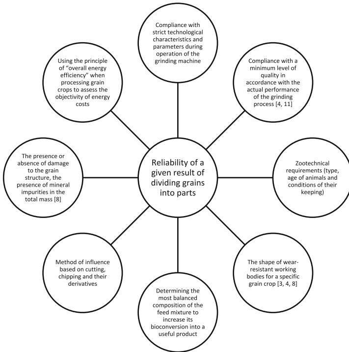
Fig. 4. Scheme for forming the reliability of the process of separating grain into a given number of parts
