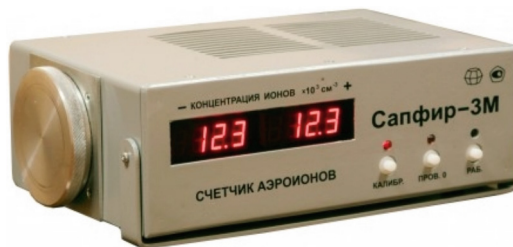
Fig. 2. The appearance of the concentration meter of positive and negative aeroions “Sapphire – 3M”
