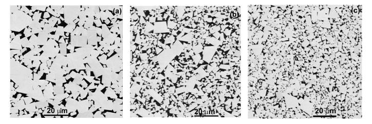
**Figure 2.** SEM micrographs of three studied samples: (**a**) WC-6 wt.% Co, (**b**) WC-11 wt.% Co and (**c**) WC-26 wt.% Co.
