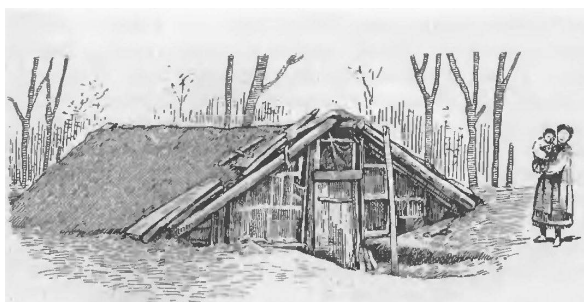
Fig. 23: Nanai xurbu , a half-dugout with gable roof (Levin and Potapov 1956: 797)
