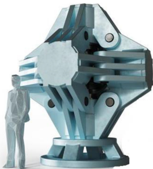
Figure 1. HPHT synthetic diamond hydraulic press.
