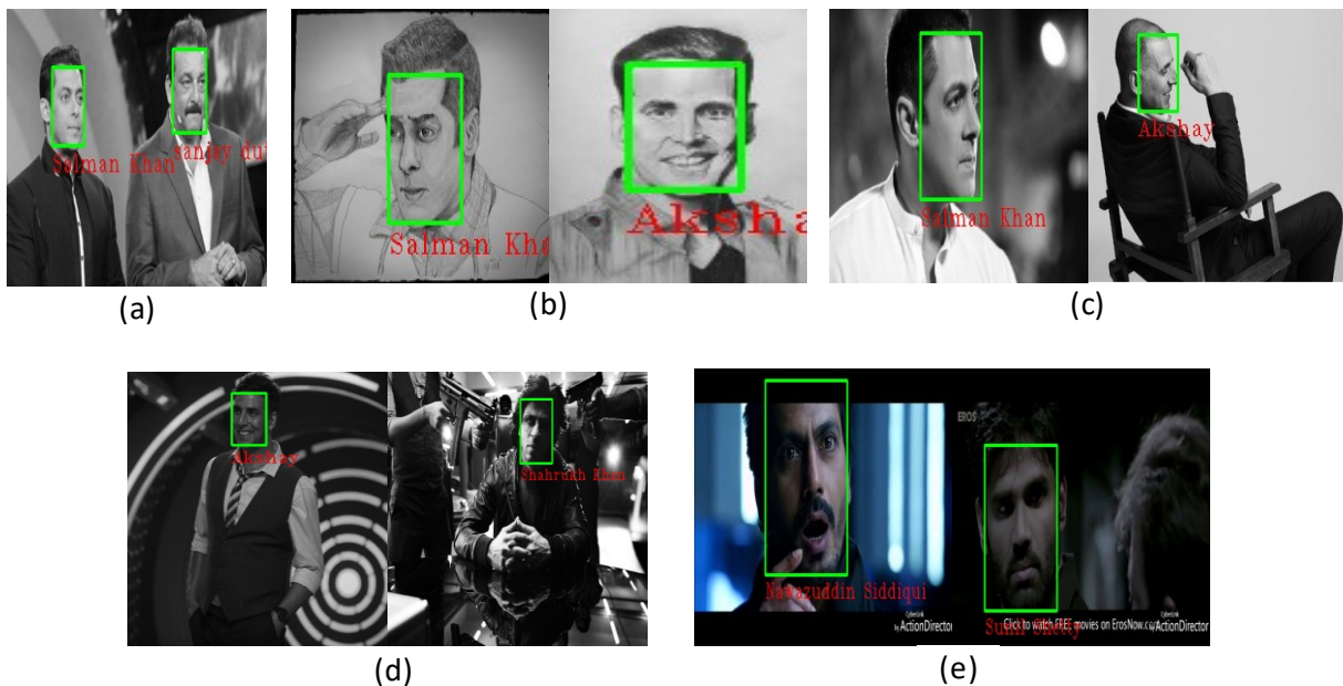
Fig. 5. Illustrate the face recognition using pretrained model i.e FaceNet. Fig. 5 (a) shows face recognition with real images, (b) shows with image drawings, (c) represents the recognition for side-face images, (d) shows recognition of face even with less light intensity and (e) recognizes from video even with dark background.
