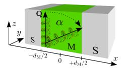
**Figure 4.** The Josephson junction configuration we consider. A spiral alignment of magnetic moments in the magnet M between the superconductors S, can be switched to uniform magnetization.
