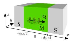
**Figure 1.** The Josephson junction configuration we consider. A spiral alignment of magnetic moments in the magnet M between the superconductors S, can be switched to uniform magnetization.
