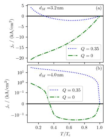
**Figure 3.** Critical current density  $j_c$  as a function of T for  $d_M = 3.2$  nm in (a) and for  $d_M = 4$  nm in (b). These figures show that one can also use the temperature T to tune our proposed device into a regime, where the critical current at the spiral magnetization has a positive sign (0 state), while the sign of the critical current in the saturation at Q = 0 is negative ( $\pi$  state).
