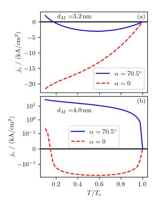
**Figure 7.** Critical current density  $j_c$  as a function of T for  $d_{\rm M}=3.2$  nm in (a) and for  $d_{\rm M}=4$  nm in (b). These figures show that one can also use the temperature T to tune our proposed device into a regime, where the critical current in the case  $\alpha=70.5^{\circ}$  has a positive sign (0 state), while the sign of the critical current in the case  $\alpha=0$  and the homogenous ferromagnet case Q=0 is negative ( $\pi$  state).
