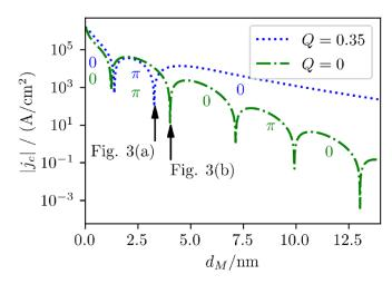
**Figure 2.** Critical current density  $|j_c|$  as a function of  $d_M$  calculated from equation (7) in the case of in-plane spiral magnetization Q=0.35 and in the homogeneous ferromagnetic case Q=0, corresponding to two logical states of the proposed Josephson SSV. For two working points  $d_M$  indicated by arrows, we show the critical current density as a function of the temperature T in figure 3.
