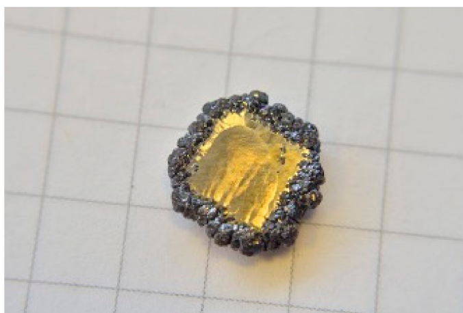
Figure 6. An M-CVD diamond with a polycrystalline jacket.
