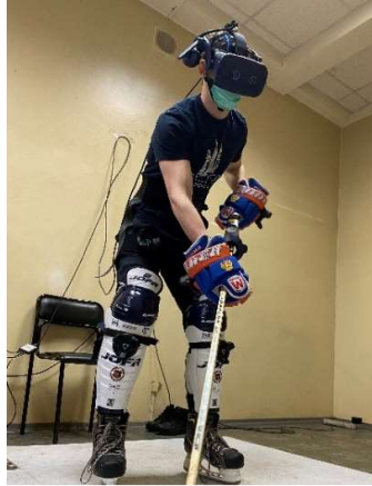
Figure 4. Subject with the trackers attached to his shin guards, hips, chest, gloves and stick
