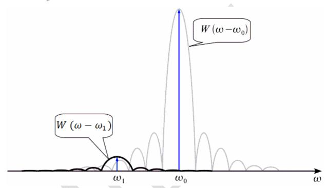
Figure 7. The smaller amplitude signal is lost in the side lobes
