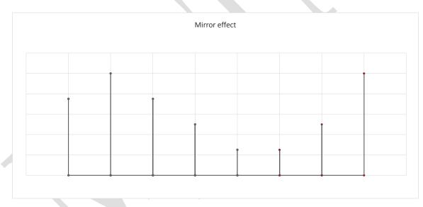
Figure 3. Mirror effect, under Fourier transform
