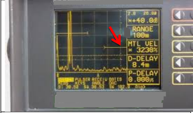
Fig.2. Display of calibration parameters for UT of castings
