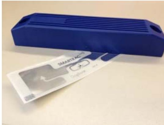
Figure 2: Comparison of size between a passive and active RFID tags
