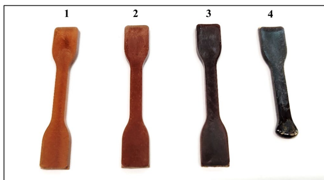
FIGURE 3 | Samples of polyimides with different molecular weights prepared by injection molding: 1—RBAPB 93, 2—RBAPB 95, 3—RBAPB 97, and 4—RBAPB 98.
