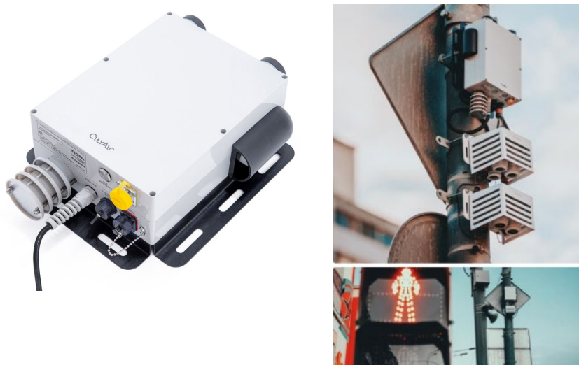
Fig. 3. The external appearance of the device for measuring microclimate values.
