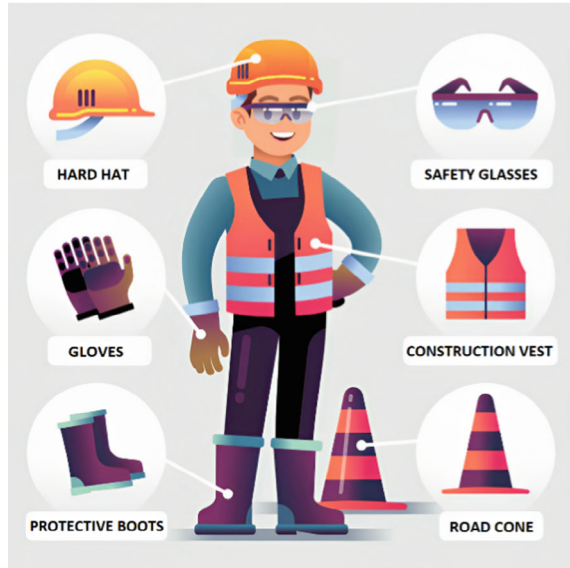
Fig. 1 Personal protective equipment spectrum: helmets to accessories (essential gloves, cones, safety glasses, protective boots, and vests)
