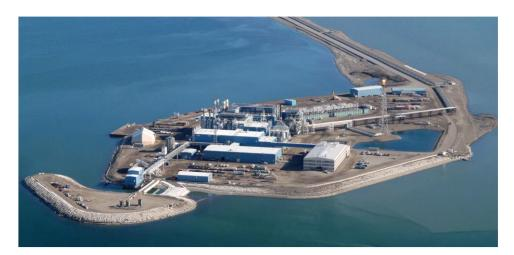
Figure 6. Endicott project of artificial gravel island
