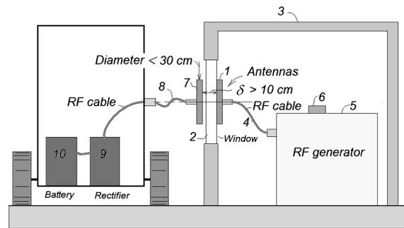
Fig. 4. Schematic of the wireless charging.
