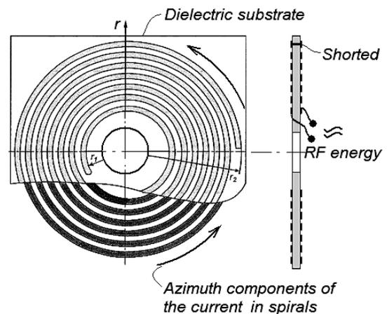
Fig. 2. Coupled arithmetic spirals on the dielectric substrate.
