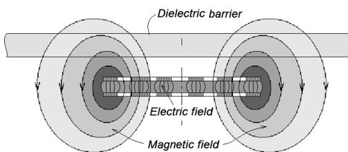
Fig. 3. Electric and magnetic fields distribution in coupled spirals.
