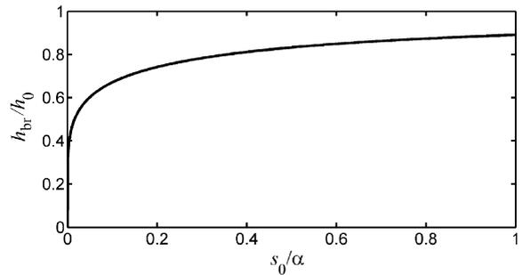
Fig. 2. Breaking depth versus wave steepness.
