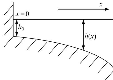
Fig. 3. The geometry of wave runup on the wall.
