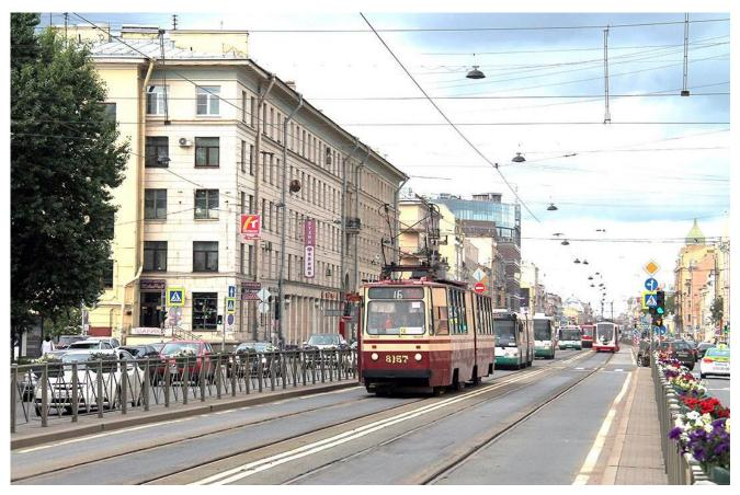
Fig. 5.2. Priority lane for buses and trams in the center of the roadway (Ligovskiy prospect).
