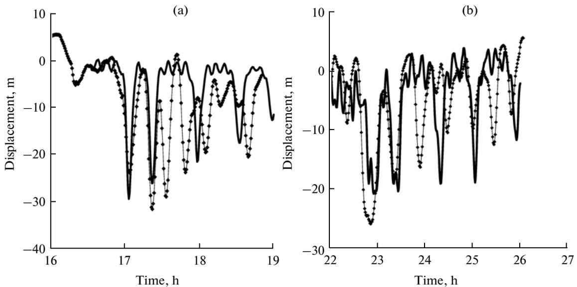
**Fig. 5.** Comparison of the modeling results (solid line) with the data of observations (dots) at points (a) 15 and (b) 16 when the coefficient of bottom friction is 0.0006.
