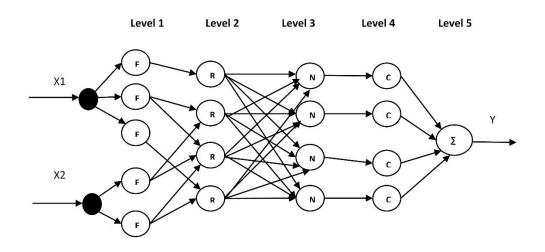
Figure 2. Architecture of ANFIS hybrid model [12]
