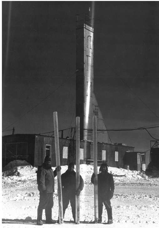
Figure 3. Cores extracted by means of TBZS-152 (33 SAE).
