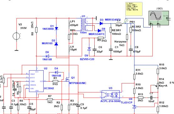
Fig. 4. Schematic diagram of pulsed SPS in Multisim PC
