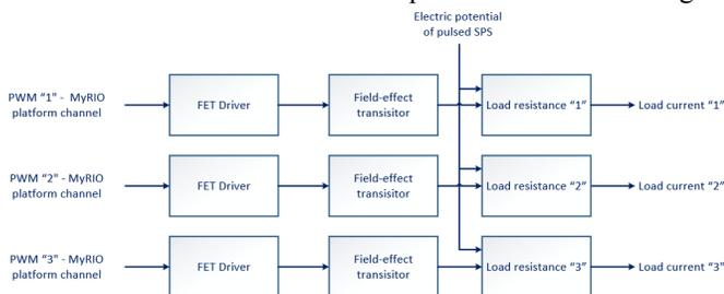
Fig. 3. Structure of the equivalent of electrical load.
