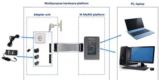
Fig. 1. Structure of the monitoring system for the parameters of pulsed SPS laptops.
