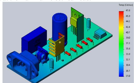
Fig. 5. Temperature distribution on the board assembly of a pulsed SPS laptop in a steady heat process at the maximum electrical load.
