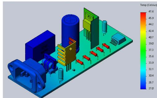
Fig. 5. Temperature distribution on the board assembly of a pulsed SPS laptop in a steady heat process at the maximum electrical load.
