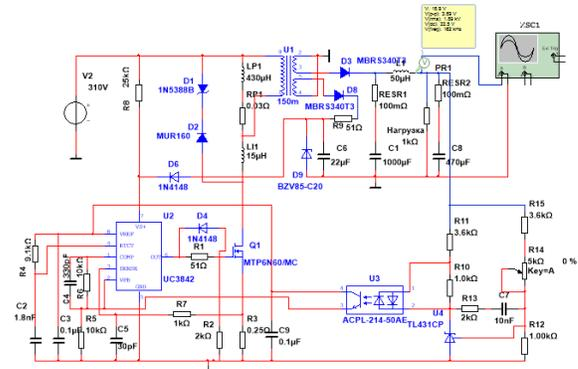
Fig. 4. Schematic diagram of pulsed SPS in Multisim PC
