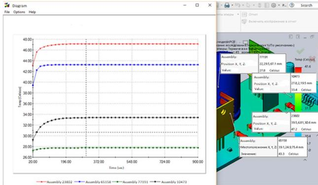
Fig. 6. Dependence of temperature at certain points of the SPS board assembly against time at the maximum electrical load.
