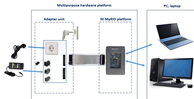
Fig. 1. Structure of the monitoring system for the parameters of pulsed SPS laptops.
