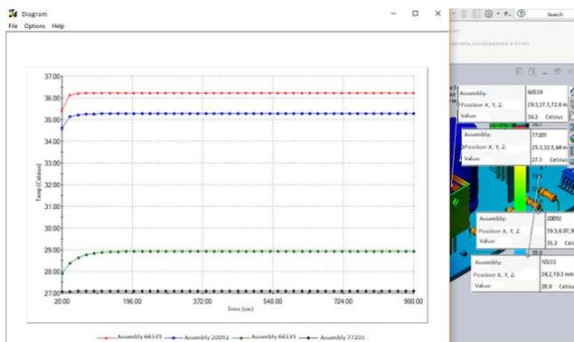
Fig. 7. Dependence of temperature in certain points of the SPS board assembly on time at a load 4 times less than the maximum.
