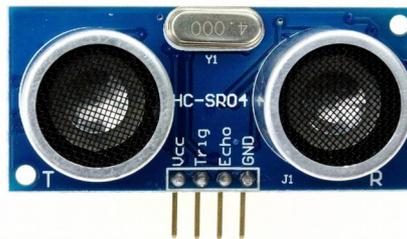
Figure 24. HCSR04 device for ultra-sonic ranging measurement.
