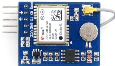
Figure 12. U-blox NEO 6-M GPS receiver module.
