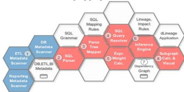
**Figure 1** Impact Analysis system architecture components.
