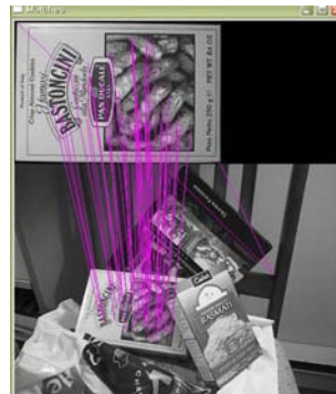
Fig. 2. Key points detection and matching using SIFT method
